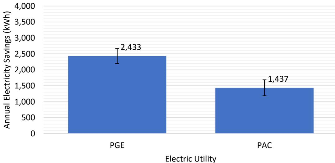
*Chart 3: Electric savings for heat pump conversions in site-built homes by electric utility*
