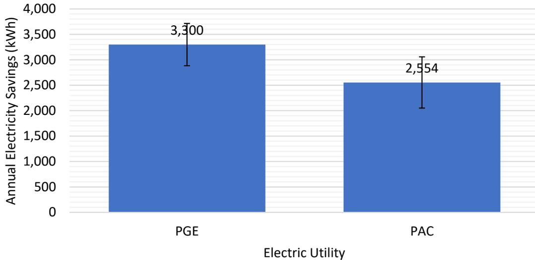
*Chart 4: Electric savings for heat pump conversions in manufactured homes by electric utility*
