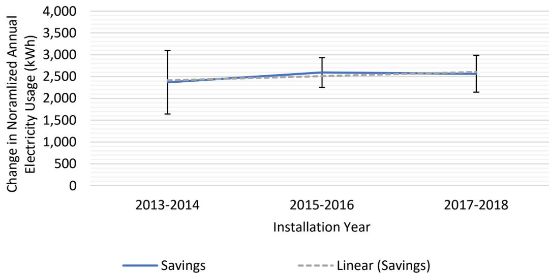
Chart 11: Electric savings for heat pump conversions in manufactured homes by installation year, 2013-2018
