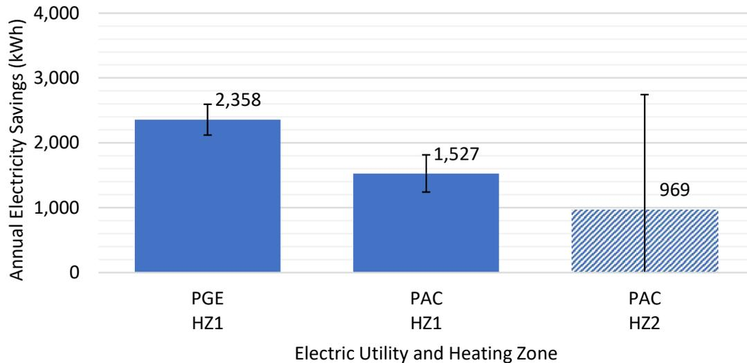
Chart 5: Electric savings for heat pump conversions in site-built homes by electric utility & heating zone<sup>6</sup>
