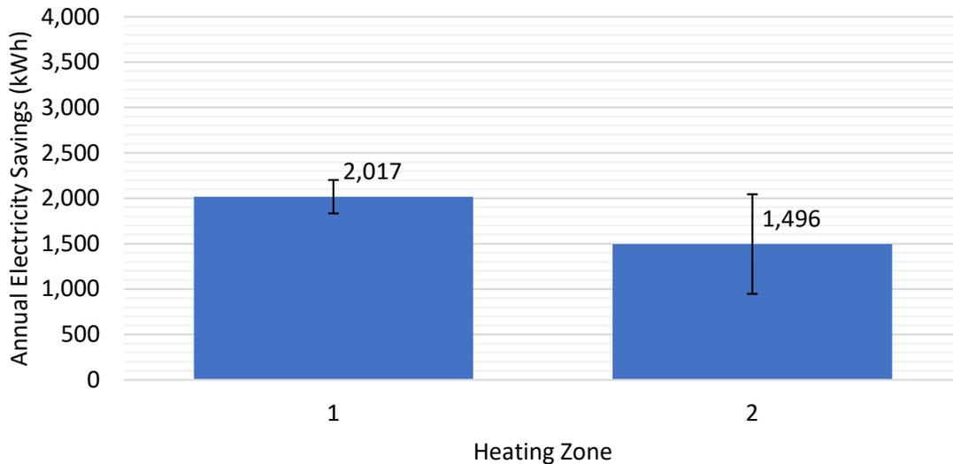
*Chart 1: Electric savings for heat pump conversions in site-built homes by heating zone*
