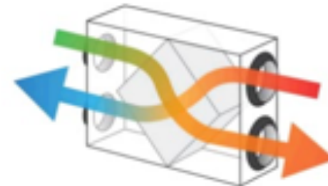
heat recovery ventilators
