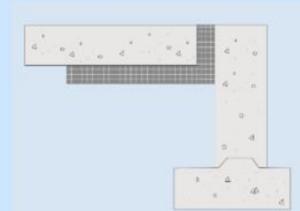
Insulation Beneath Slab— Not permitted
